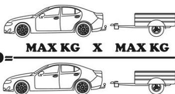
$$D = \frac{\text{MAX KG} \times \text{MAX KG}}{\text{MAX KG} + \text{MAX KG}} \times 0,00981 \leq 15,2 \text{ kN}$$
